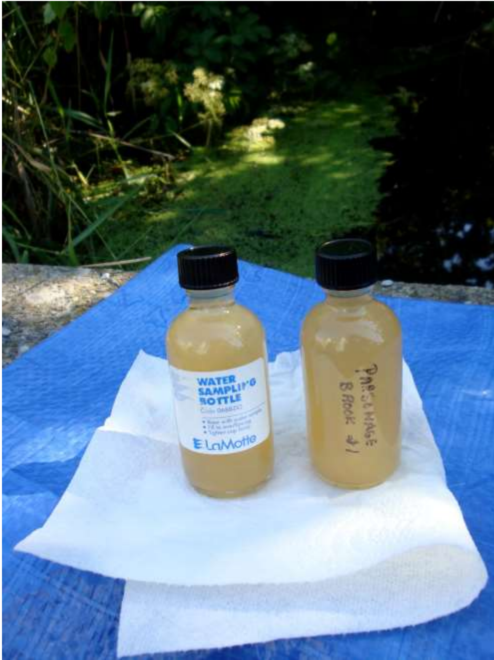
4441 bottles for dissolved oxygen testing (waiting for flocculant to settle before final "fix")
